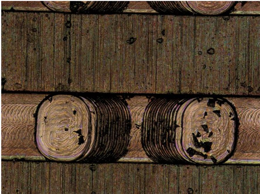
*Figure 18 Scanning Laser Image of 400µm Microchannel with Notches Chip 10x magnification*
