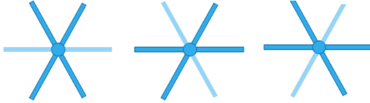
Figure 11: Phantom Network Unit Cell . Our construction is based off of a standard ordered triangular lattice, whose unit cell is illustrated in Figure 4. For each node, randomly two of the three filaments present are crosslinked, and the third filament simply passes through the connection. Because of this, the third filament does contribute to the deformation energy of the network as a whole, but is not visible when viewing only the unit cell (detailed later). Since the third filament is physically there, however for all intents and purposes cannot be seen by the rest of the unit cell, we refer to it as a "phantom". The three versions depicted represent the three possible unit cells which arise.
