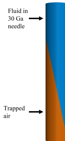
Figure 6.1. Fluid in a 12^\circ beveled non-coring 30 Ga needle and trapped air between it and the septum. The trapped air can introduce air bubbles to the system as big as 7.5 nL.
