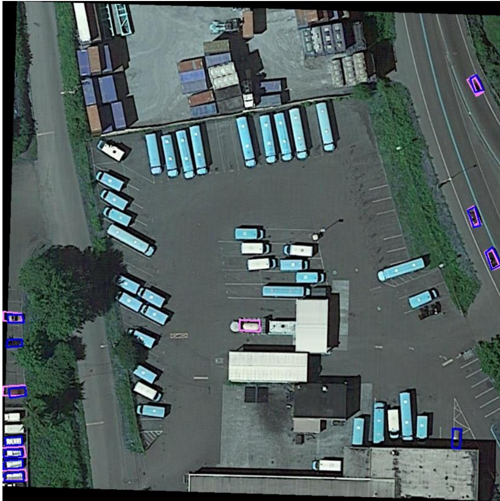
Fig 11.6 Detection visualization for Deformable YOLO. The pink boxes are detections while blue circles are ground truth. The network predictions are not restricted to rectangles or squares as can be seen in the top right car images.
