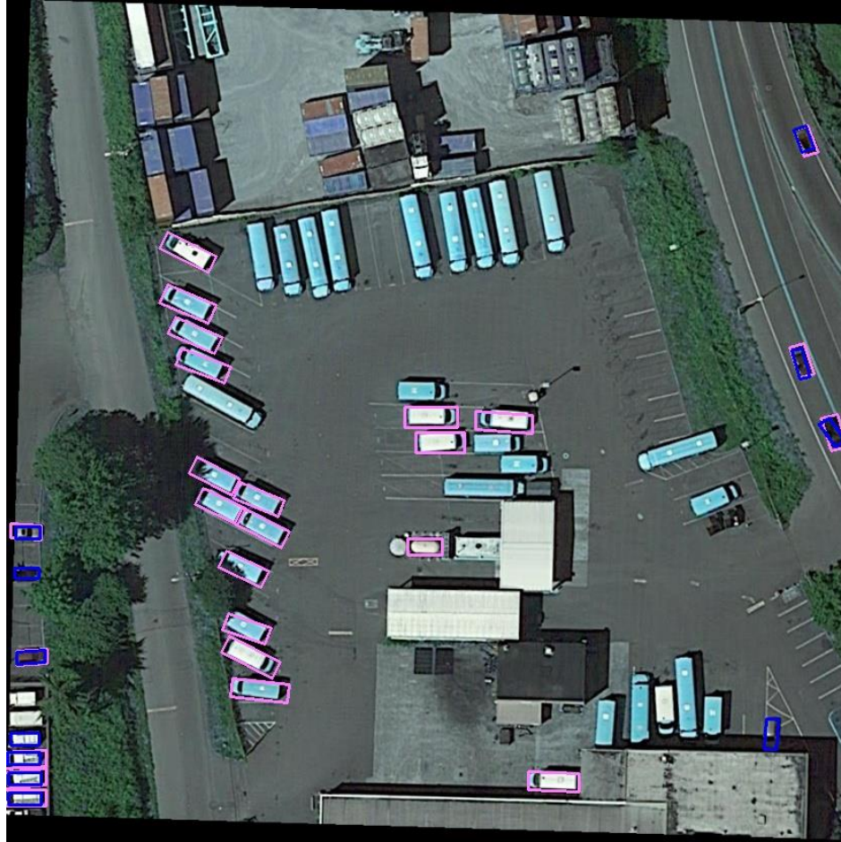
Fig 11.4 Detection visualization for YOLO v3, with +/- 45-degree rotation. The pink boxes are detections while blue circles are ground truth. The network detects large vehicles as small vehicles which leads to lower scores
