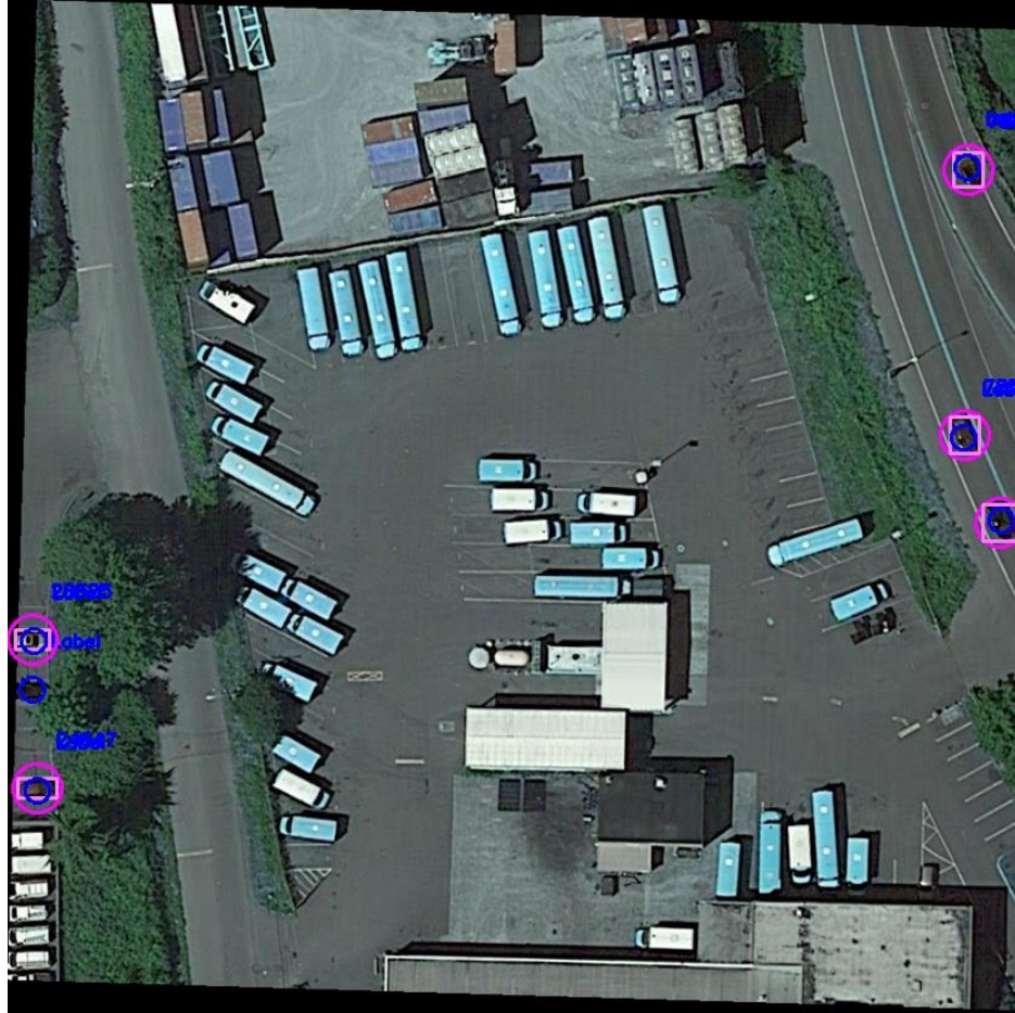
Fig 11.1 Detection visualization for YOLO v3, without any rotation. The pink box and circles are detections while blue circles are ground truth.
