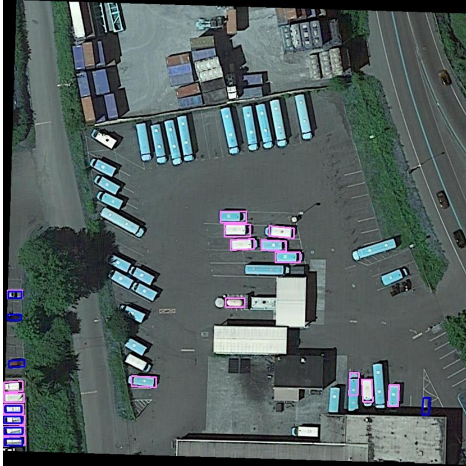
Fig 11.2 Detection visualization for YOLO v3, with +/- 10-degree rotation. The pink boxes are detections while blue circles are ground truth. Note the mistaken identifications which contributed to low scores.
