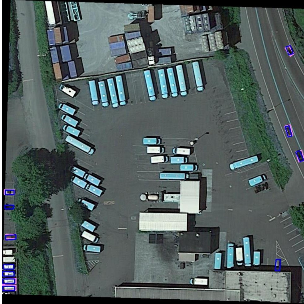
Fig 11.5 Detection visualization for YOLO v3 Extra Anchors. The pink boxes are detections while blue circles are ground truth. The network accurately detects objects of all rotations.
