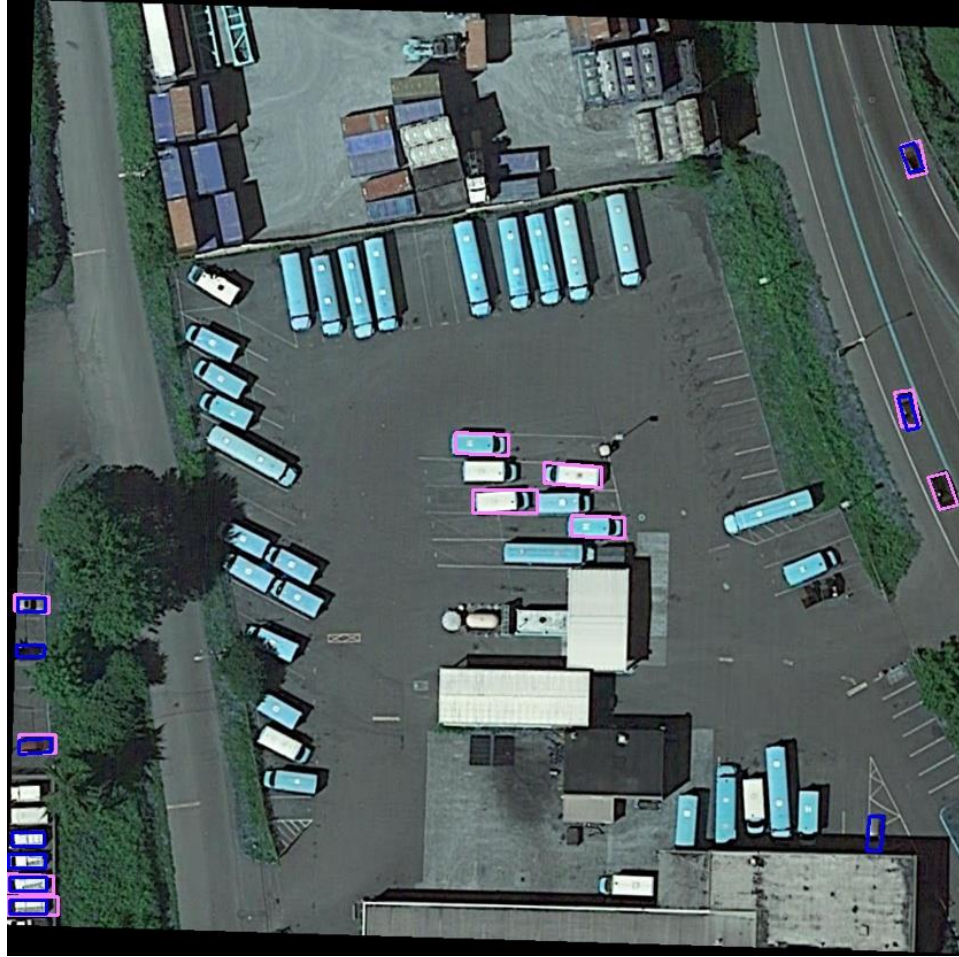
Fig 11.3 Detection visualization for YOLO v3, with +/- 25-degree rotation. The pink boxes are detections while blue circles are ground truth. The network detects objects that are rotated by almost +/- 25 degrees, giving false predictions.
