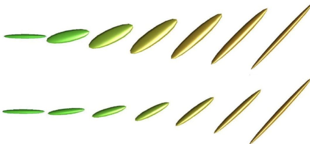
Figure 5: Interpolation between two tensors, which can be thought of as a template tensor (far left) and a reference tensor (far right). Top: linear interpolation. Bottom: Log-Euclidean interpolation. Note the swelling that occurs in the case of linear interpolation. Taken from [10].
