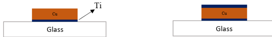
Figure 4.1: (a) Ti/Cu and (b) Ti/Cu/Ti gate metal film stacks employed to investigate copper electrode adhesion and copper diffusion effects on the gate dielectric and IGZO channel.
