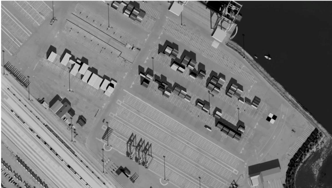
Figure 2.16: DIRSIG simulation of the Port of Tacoma, WA imaged with a 2-D framing array on a commercial small satellite [149].
