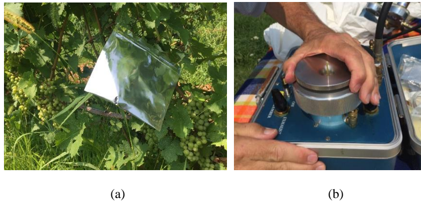
Figure 3.2. Our study used the field parameter stem water potential ( \psi_{\text{stem}} ) to directly measure vine water content at time of flight. (a) Leaves were bagged for at least 30 minutes prior to flight to allow for equilibration of leaves with vine plant; (b) A pressure chamber was used to capture real-time \psi_{\text{stem}} for 56 individual vine plots
