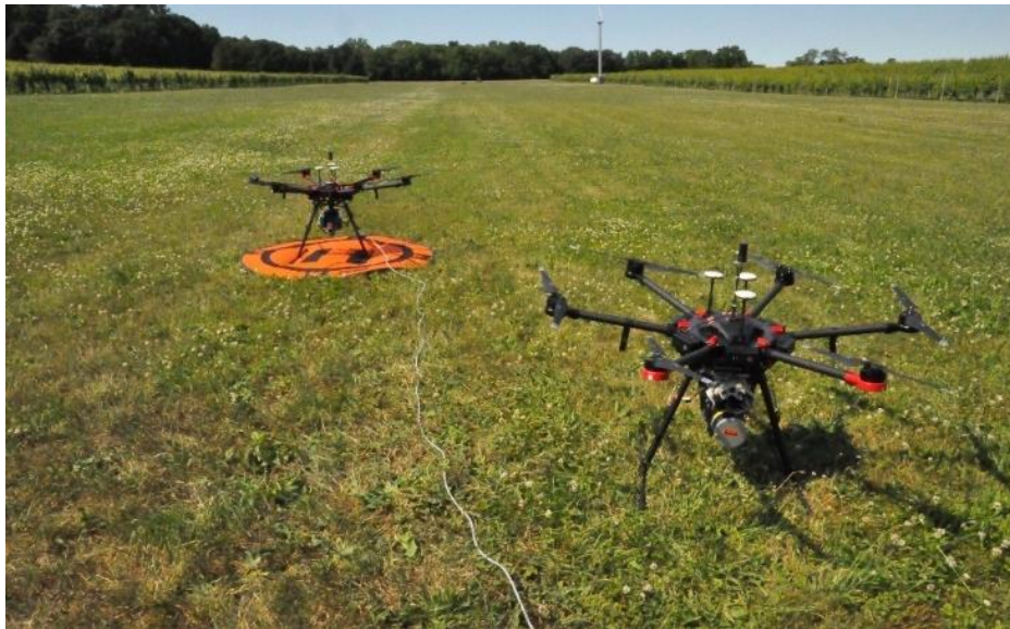
Figure 4.3. Two separate multi-copter platforms were employed in our air campaign efforts. Both multi-copter designs exploited the modular DJI Matrice 600 flying platform. One of the multi-copters was equipped with a VNIR imaging sensor, while the other was equipped with a SWIR imaging sensor; both sensors boasted high spectral resolution – hyperspectral – sensors provided by Headwall Photonics (Izzo et al. 2019).
