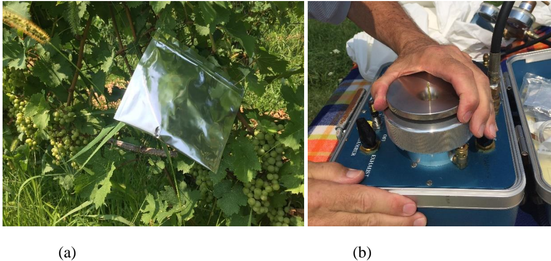
Figure 4.4. A PMS Model 600 Pressure Chamber Instrument was used to capture the real-time traditional field measurement of \psi_{\text{stem}} during time of flight. Leaves were placed inside of aluminum bags before measurement to allow for assessment of integral plant water status (a) and then inserted into the pressure chamber instrument for measurement of \psi_{\text{stem}} (b) (Izzo et al. 2019)
