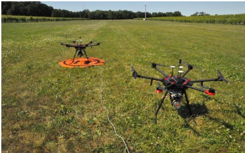
Figure 3.1. Our study used two Matrice 600 multi-copters, both equipped with Headwall hyperspectral imaging sensors. One of the on-suite sensors covered the VNIR regime from 400-1000 nm, while the other covered the SWIR regime from 1000-2500 nm. We focused on initial analysis of the VNIR flights in this manuscript.
