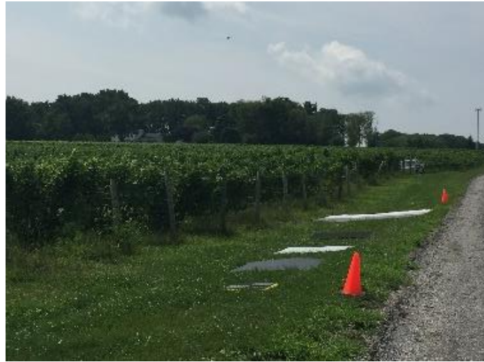
Figure 3.3. We used the established 2-Point ELM to convert our imagery to reflectance. Around time of flight, we captured known reflectance curves of in-scene calibration panels, light and dark, via an SVC spectroradiometer.
