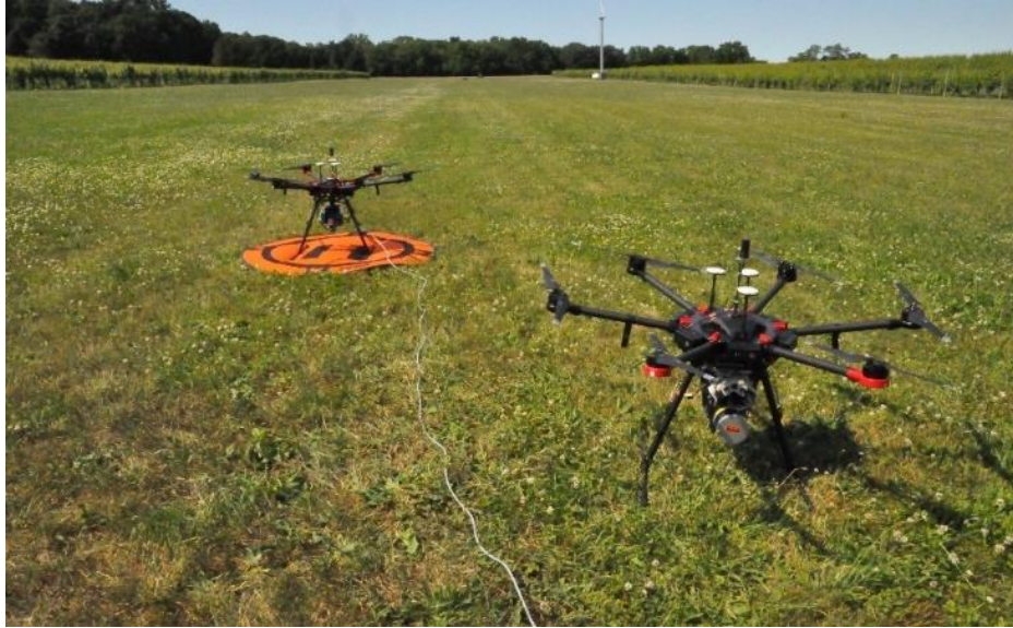
Figure 2.1. Two separate multi-copter platforms were employed in our air campaign efforts. Both multi-copter designs exploited the modular DJI Matrice 600 flying platform. One of the multi-copters was equipped with a VNIR imaging sensor, while the other was equipped with a SWIR imaging sensor; both sensors boasted high spectral resolution – hyperspectral – sensors provided by Headwall Photonics
