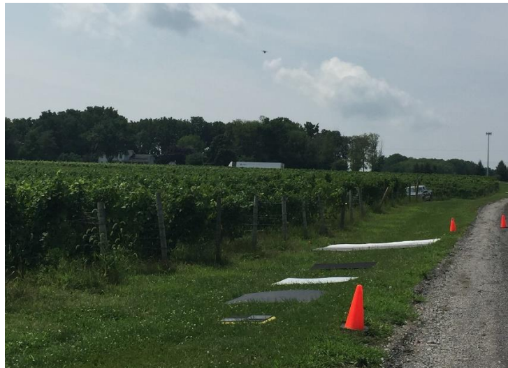
Figure 4.5. We normalized all of our captured imagery to the reflectance space so that we could justifiably make direct comparison of all of our flight data across multiple days of flight. We placed in-scene calibration panels during all flights, and captured associated reflectance curves using an SVC spectrometer, to perform this normalization via the 2-point ELM (Izzo et al. 2019).
