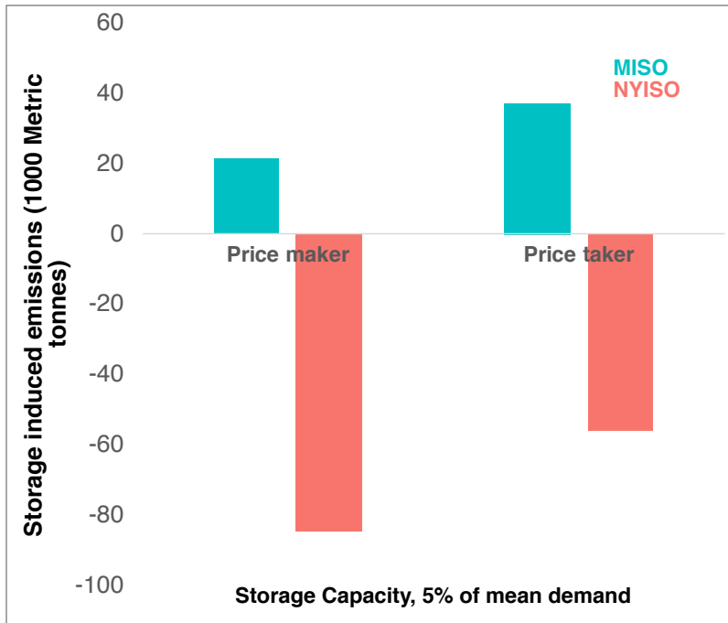
Fig. 21 Difference in annual storage induced emissions when large capacities of storage are considered a price-taker instead of price-maker in New York ISO (NYISO) and Midcontinent ISO (MISO). The storage capacity considered is 5% of the average demand, which is 12GW in MISO, and 4GW in NYISO. The estimated storage-induced emissions are given in metric kilo tonnes of CO 2eq . The colors of the bars indicate the ISOs. Price-taker scenario over-estimates the annual storage induced emissions in MISO by 75% and in NYISO by 35%.
