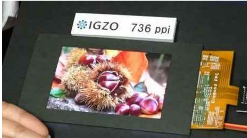
Fig 5. Sharp Develops IGZO 4K Ultra HD Screen with Stunning Pixel Density of 736ppi [6]
