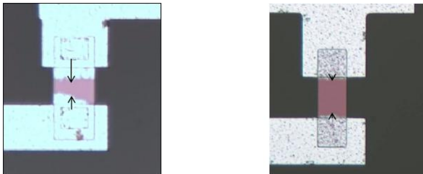
Fig. 21. Al encroachment from source/drain regions into silicon channel. As observed, the encroachment via contact cut is much more than the other case where S/D metal is in direct contact with silicon mesa. (L/W = 24/24 and 48/24 respectively)
