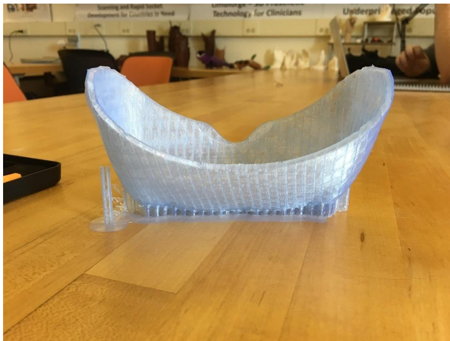
Figure 12: Test print with brim and supports. Pieces of excess material are printed on the bottom of the base (brim), as well as going up from the brim to support the print (supports). These pieces are broken off after printing and discarded. Image courtesy of author.
