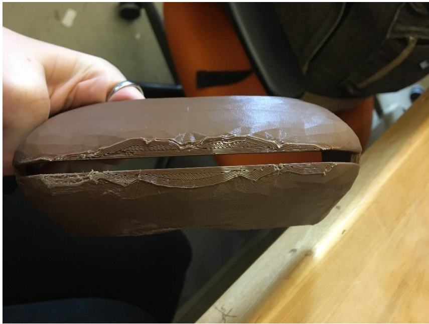
Figure 19: Visor after brim was removed. Not all of the brim could be removed, as part of it made up the edge of the visor. This edge was later sanded and painted so as to not stand out. Image courtesy of author.
