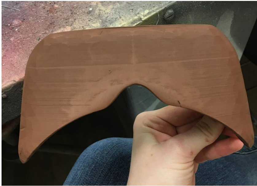
Figure 23: Completed model of the snow visor. After the airbrush process was done, the final print of the visor was completed. The paint did not completely fix the discoloring caused by sanding, however, it was even enough to be acceptable for testing. Image courtesy of author.
