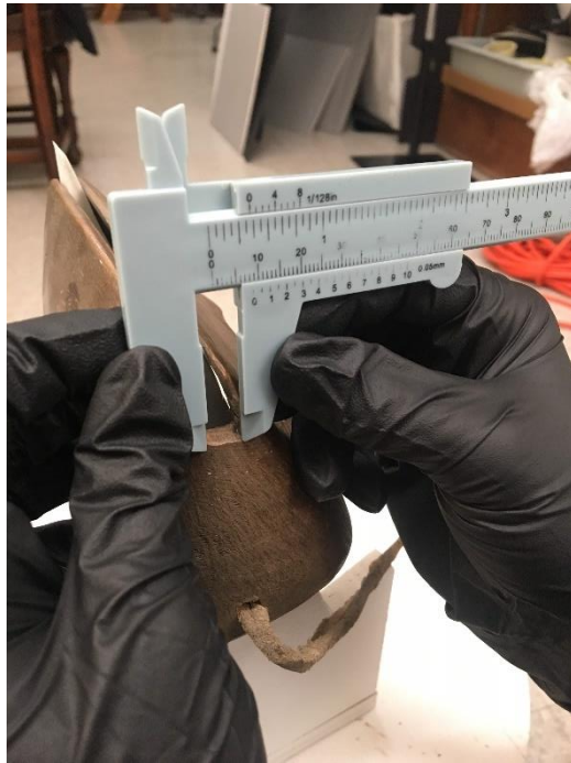
Figure 7: Snow visor being measured. Using calipers, different parts of the visor were measured after the scanning process was completed. This allowed for the scale of the visor to be checked once the models were made. Image courtesy of Jade Myers.
