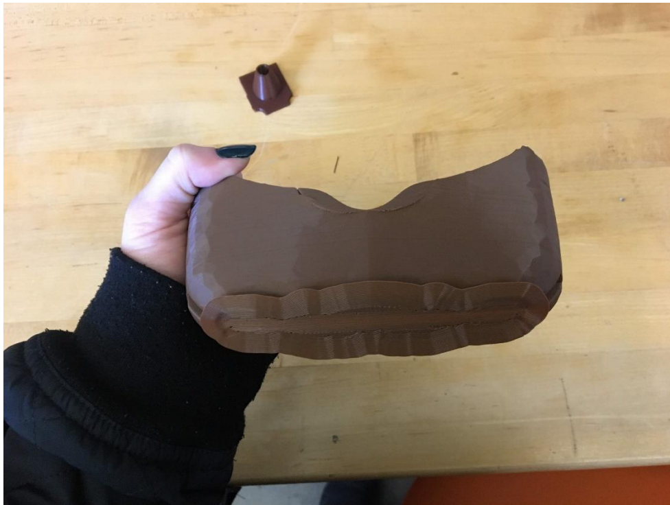
Figure 18: Brim on the final print. The excess material at the bottom of the print needed to be removed, as it was only there to provide support during printing. It was removed first with pliers, then a chisel, and finally with sandpaper. Image courtesy of author.
