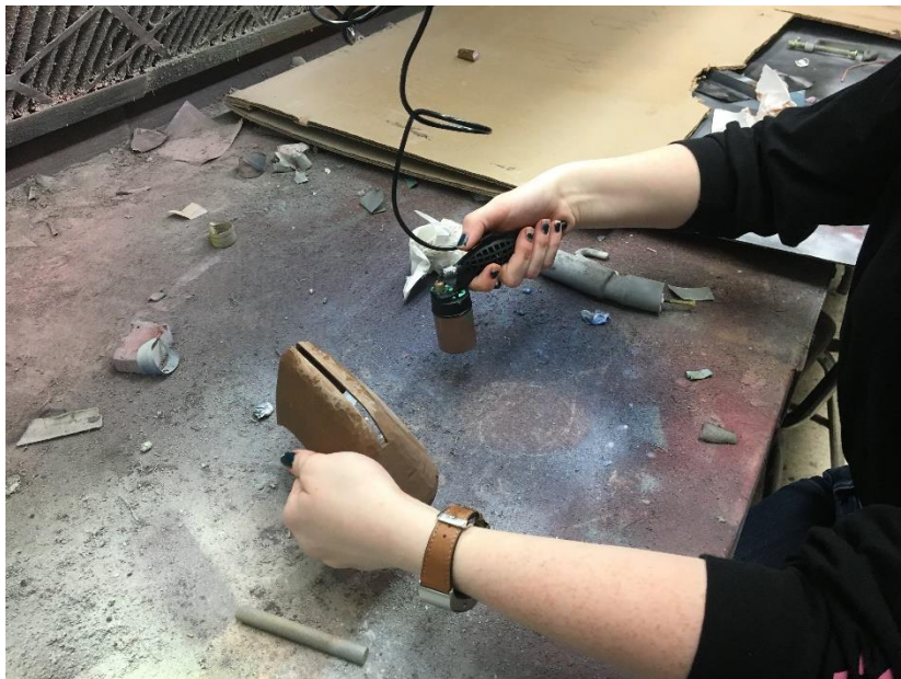
Figure 22: Author airbrush painting the model. The visor was airbrush painted brown after the sanding process to even out the color. Inadvertently, this also made the print look and feel more like wood, the material of the original visor. Image courtesy of John Lyons.
