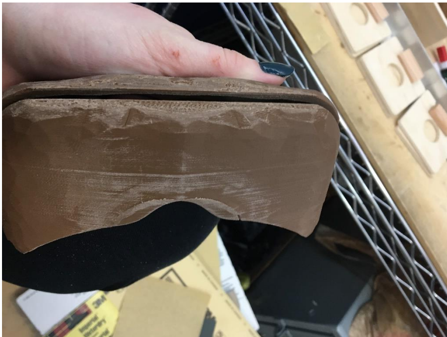
Figure 20: Visor during sanding process. Physical defects such as uneven areas, sharp edges, and the excess brim were removed with sanding. Image courtesy of author.
