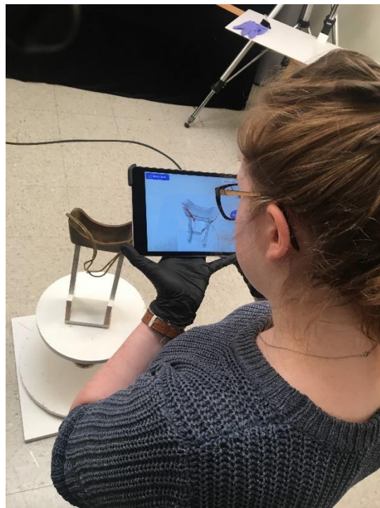
Figure 6: Author scanning the visor. The visor was scanned using a Structure Sensor iPad attachment. The model of the scanned visor appears in white on the iPad screen. Image courtesy of Jade Myers.
