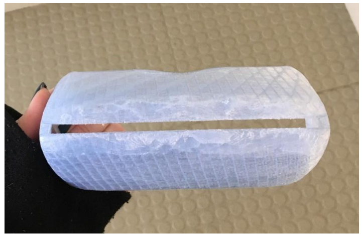
Figure 16 and Figure 17: Second test print after printing. The second test print was much closer in size to the original visor, and the nose hole was a much better shape. Both images courtesy of author.
