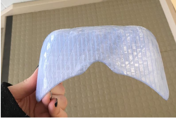
Figure 16 and Figure 17: Second test print after printing. The second test print was much closer in size to the original visor, and the nose hole was a much better shape. Both images courtesy of author.
