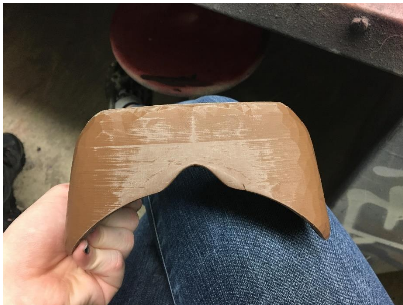
Figure 21: Visor after sanding process. The sanding process removed many of the physical defects that the print had, but also discolored the sanded areas. Image courtesy of author.
