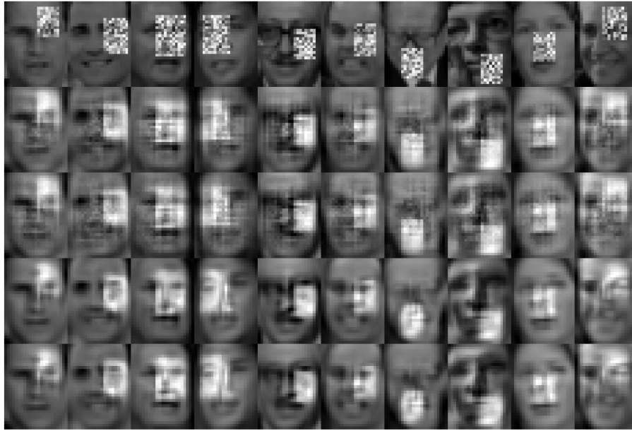
Figure 4.26: Reprojection of face images using the proposed PM-L_1 -PCA and standard L_2 -PCA principal components extracted from the corrupted face training set. First row: Input Image. Second row: Reprojection using L_2 -PCA. Third row: Reprojection using PM-L_1 -PCA with Reprojection Minimization Formulation. Fourth row: Reprojection using PM-L_1 -PCA with Projection Maximization Formulation. Fifth row: Reprojection using PM-L_1 -PCA-W with Projection Maximization Formulation.
