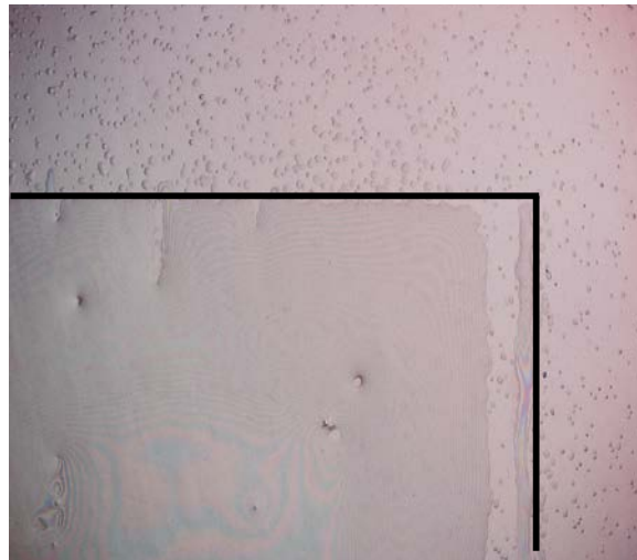
Figure 41. One cm square, inkjet printed Optimized PZT sol-gel on a polished stainless-steel substrate (500 \mu\text{m} scale).
