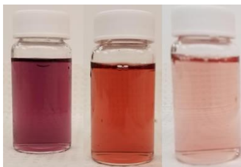
Figure 26: A tris(maltonato)iron(III) solution was adjusted to pH 2 using HCl (left), adjusted to pH 4 with NaOH (middle), the same sample adjusted back to pH 2 with phosphoric acid (right).
