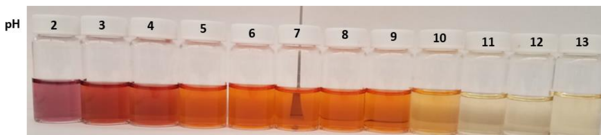
Figure 23: Range of standard iron (III) maltol complexes at different pH's adjusted with HCl and NaOH
