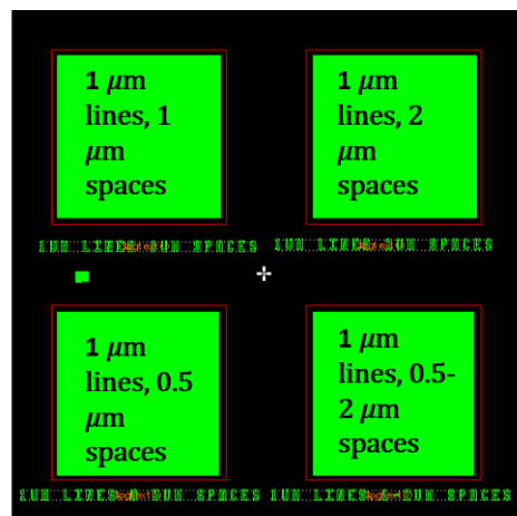
Figure 6.1: Designs of passive modulator. 1 \mu\text{m} lines and 1 \mu\text{m} spaces (top left), 1 \mu\text{m} lines and 2 \mu\text{m} spaces (top right). 1 \mu\text{m} lines and 0.5 \mu\text{m} spaces (bottom left). 1 \mu\text{m} lines and 0.5, 1, 1.5, 2 \mu\text{m} spaces (bottom right) where each space increment covers 1 mm of distance.
