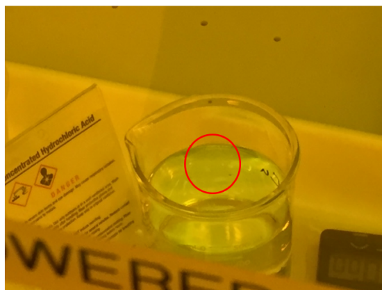
Figure 6.14: Graphene and PMMA stack floating along the surface of the Cu etchant. Blue tinge in solution is the dissolved Cu from the Cu foil.
