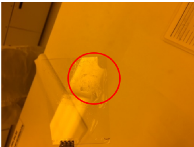
Figure 6.6: PMMA on graphene being transferred using glass slide method to maintain the integrity of the film.
