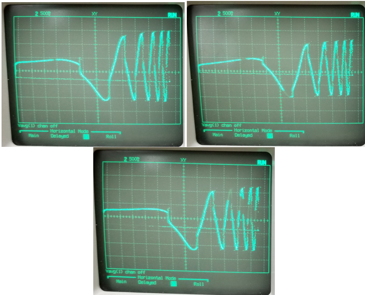
Figure 5.9: Top left: Silicon diode limiter distortion frequency sweep with XY scope. Top right: Germanium diode limiter distortion frequency sweep with XY scope. Bottom: Mixed diode limiter distortion frequency sweep with XY scope.
