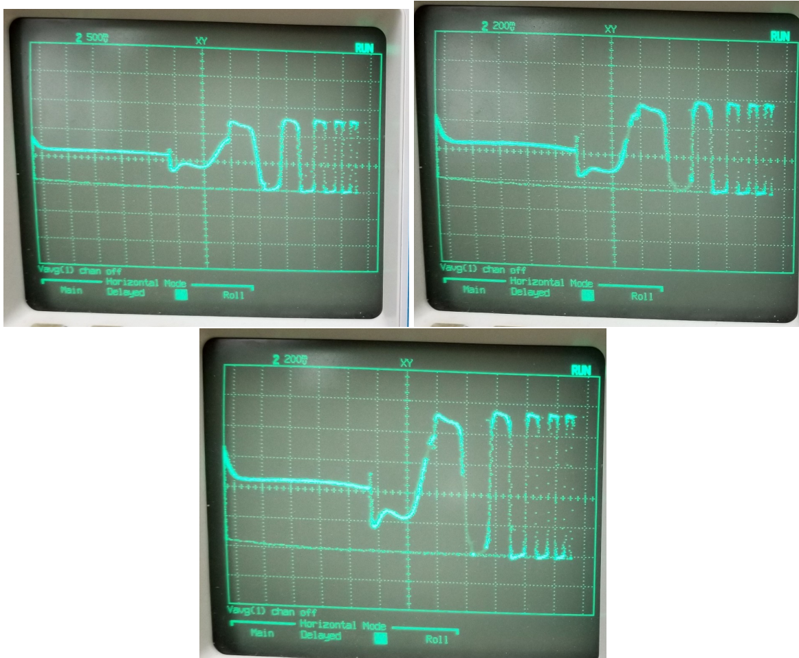
Figure 5.6: Top left: Silicon diode limiter distortion frequency sweep with XY scope. Top right: Germanium diode limiter distortion frequency sweep with XY scope. Bottom: Mixed diode limiter distortion frequency sweep with XY scope.
