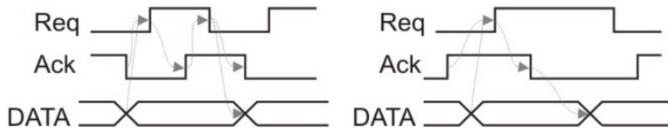
Figure 2.2: 4 phase protocol (left) and 2 phase protocol (right) [1]
