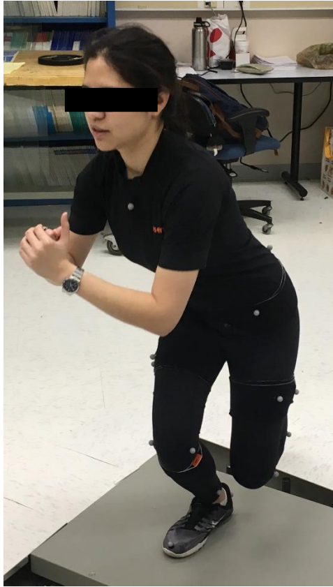
Figure 17. Subject performing a single leg squat test using the Xsens and Vicon systems.
