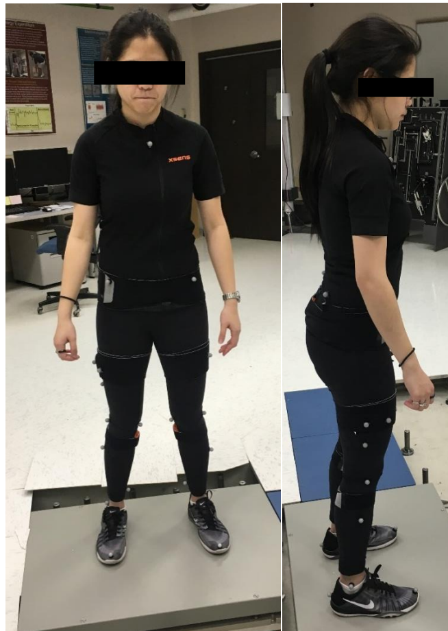
Figure 16. Front and side view of the test markers for single leg squat movement captures.
