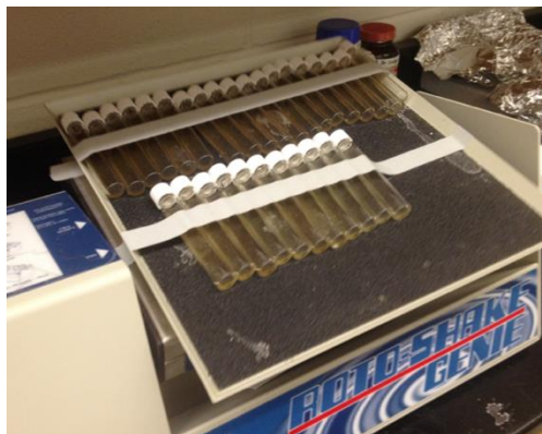
Figure 10. The n-C60 samples taken after different settling times were placed on the rotary shaker for ten minutes prior to the toluene extraction.
