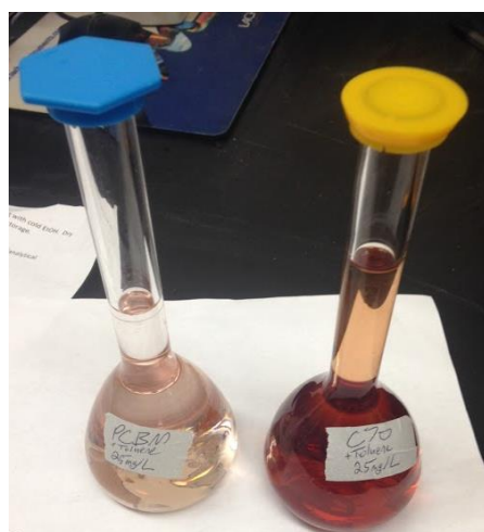
Figure 7. PCBM 25 mg/L standard (a light red color) and C70 25 mg/L standard (bright orange color) both dissolved in toluene.
