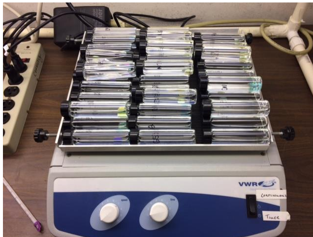
Figure 13. The set-up for the weathering of OPV cells from the University of Michigan is shown where the cells were placed into a vial with artificial freshwater (SFW) and are shaking on a shaker table at a constant speed of 1 under UV-A lighting. This experiment was started on 7/6/17 and continued for three months before adding Daphnia to test the toxicity of the weathered cells. Vials were placed randomly to eliminate bias and were randomly moved to different locations throughout the experiment to ensure all sides had exposure to UV-A light.
