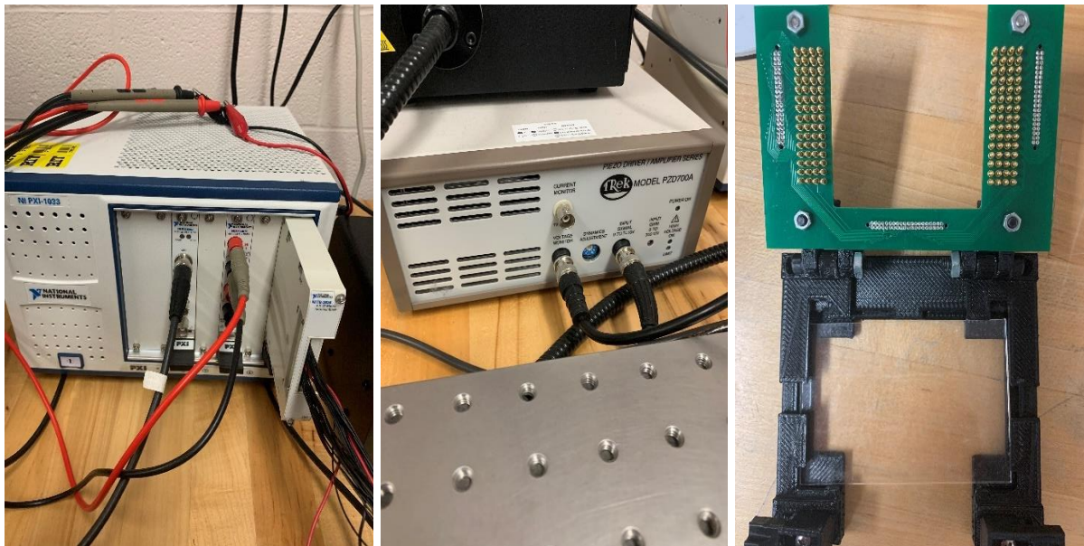
Figure 3.19: Signal generator with digital multimeter in chassis (left), voltage amplifier (middle), and pogo pin board from the Wheeler laboratory to control the DMF (right)
