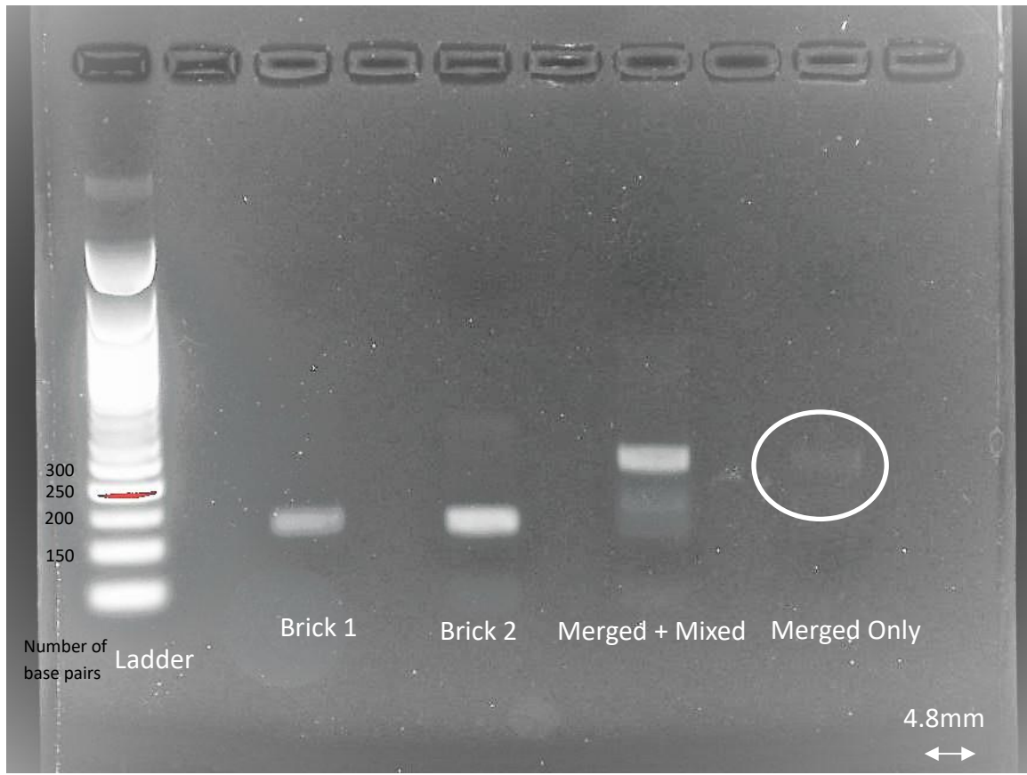
Figure 4.5: DNA Gel electrophoresis of a merged and mixed droplet on DMF device next to a merged only on DMF device
