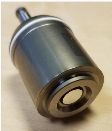
Figure 36: FDV with mirror glued to spool in assembly.
