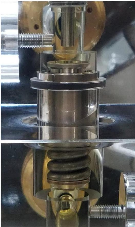
*Figure 39: FDV during data collection. Shows test pressure point with no cavitation/bubble formation.*
