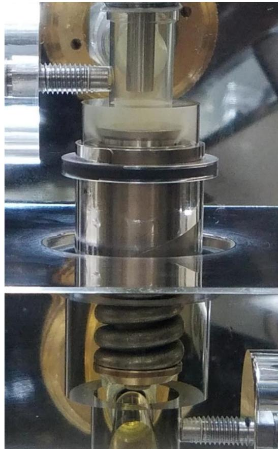
*Figure 40: FDV during data collection. Shows test pressure point with cavitation/bubble formation.*
