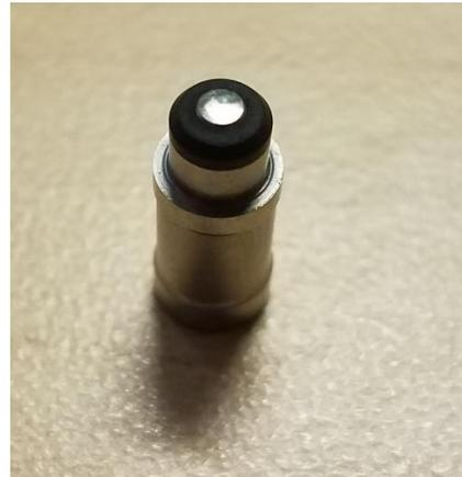
Figure 35: Mirror surface on poppet out of assembly.
