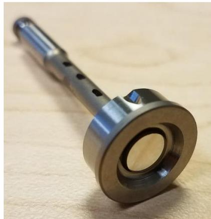
Figure 37: Mirror glued to spool out of assembly.
