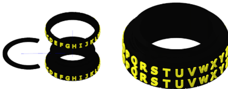
Figure 1. High contrast Caesar cipher ring with tactile feedback. The ring, comprised of two rows of enlarged, yellow letters from the English alphabet, would click when the top row was shifted.
