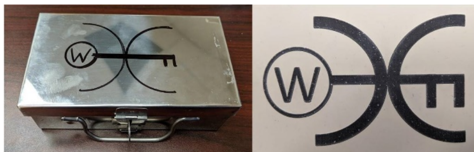
Figure 5. A metal box containing a Raspberry Pi broadcasting a WiFi network. A drawing of a symbol of a key with a 'W' in its handle and two half-circles (shown left) and a tactile graphic of the same key symbol created using a PIAF machine and swell-touch paper (shown right) were used to denote a WiFi access point.
