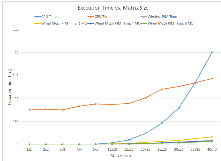
Figure 8.1: Execution time of Matrices sized between 1x1 and 40x40 for CPU, GPU, and PIM architectures.
