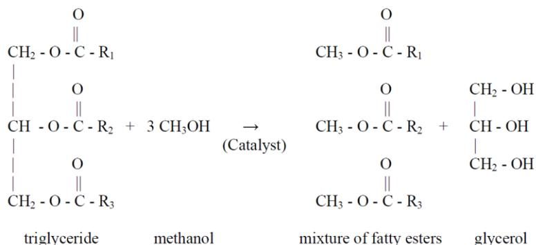
**Figure 6.10: TRANSESTERIFICATION REACTION TO BIODIESEL**
