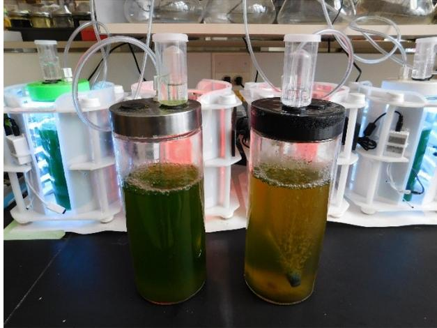
Figure 1.6 A Photo-bioreactor treatment set-up in the Lab
