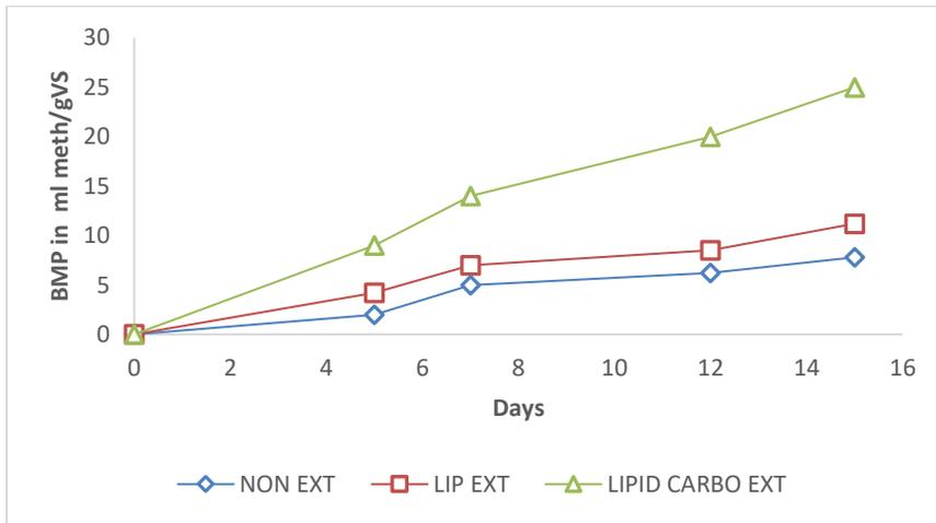
Figure 6.9 Comparing methane yield from extracted and non- extracted algae and dairy manure.
