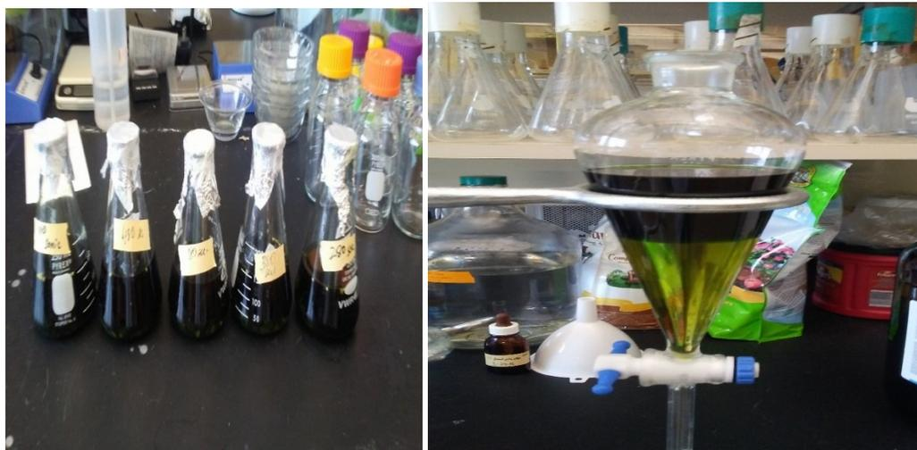
**Figure 1.9: Lipid extraction from sonicated algae biomass using organic solvents**
