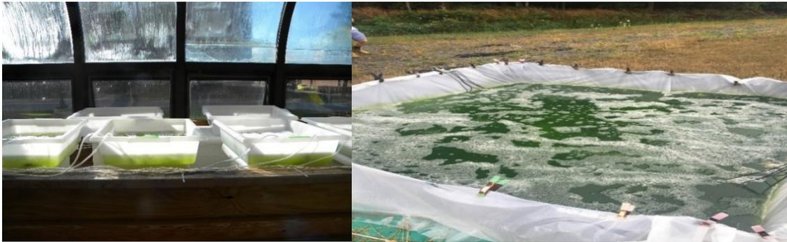
Figure 1.7 High Rate Algal Pond treatment at RIT's Green house and on-site. Treatment in a 50-gallon tank (Upper). Treatment in 15L basins (Lower left) and treatment in 1220-gal tank onsite at Synergy LLC (Lower right)
