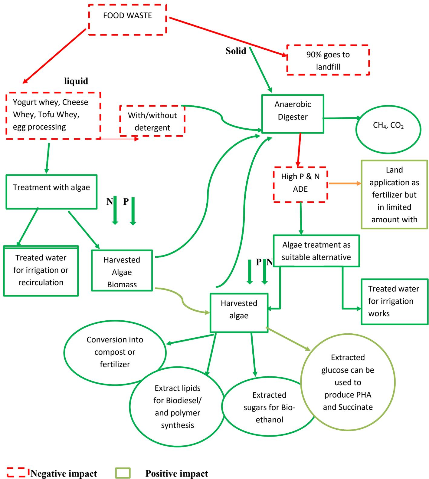
**FIGURE 7.1: THE FIGURE ABOVE DEMONSTRATES THE VARIOUS PATHWAYS FROM WASTEWATER REMEDIATION TO FINAL PRODUCTS RECOVERY.**
