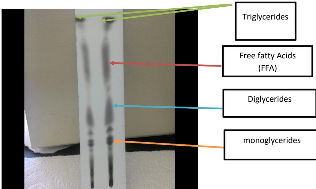
**Figure 6.1: (a) Lipid profile extracted from Chlorella sp used to treat wastewater**
