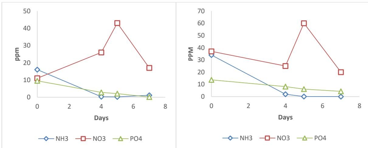
FIGURE 3.8: Nutrient reduction by isolated ADE algae on ADE and Egg wash wastewater.
