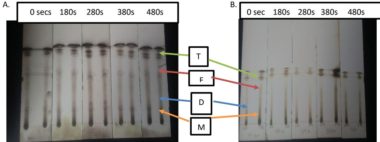
Figure 6.3 (A) TLC Chromatograms of sonicated biomass run 1
