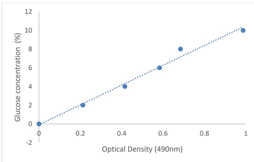
Figure 6.5 Standard curve for sugar concentration
