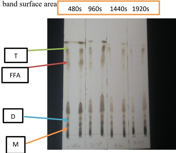
Figure 6.4 Thin layer chromatogram from increased sonication times
