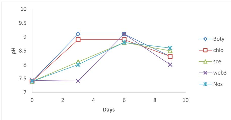
**Figure 3.3 Changes in pH during nutrient reductions of ADE by various microalgae**
