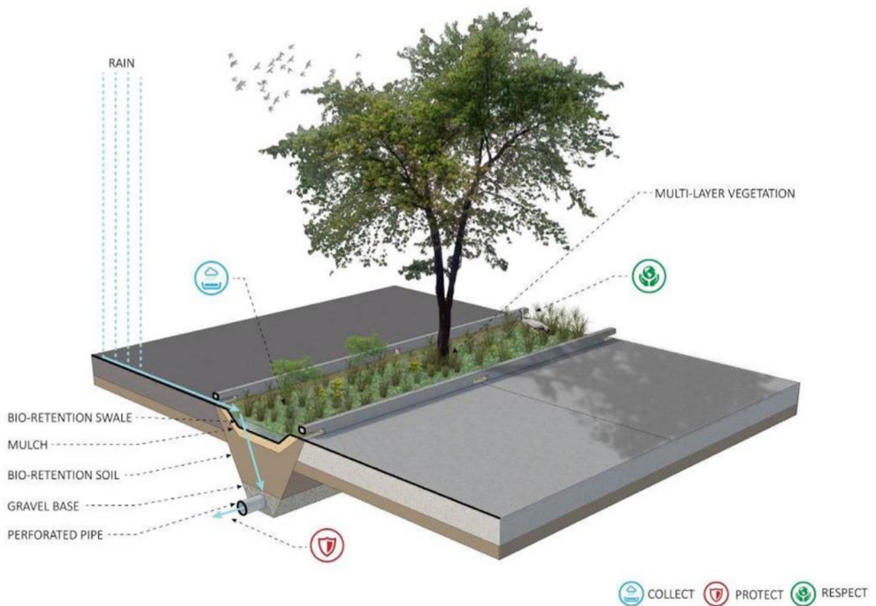
Figure 5: Bioswale, source: Jason Manongdo
