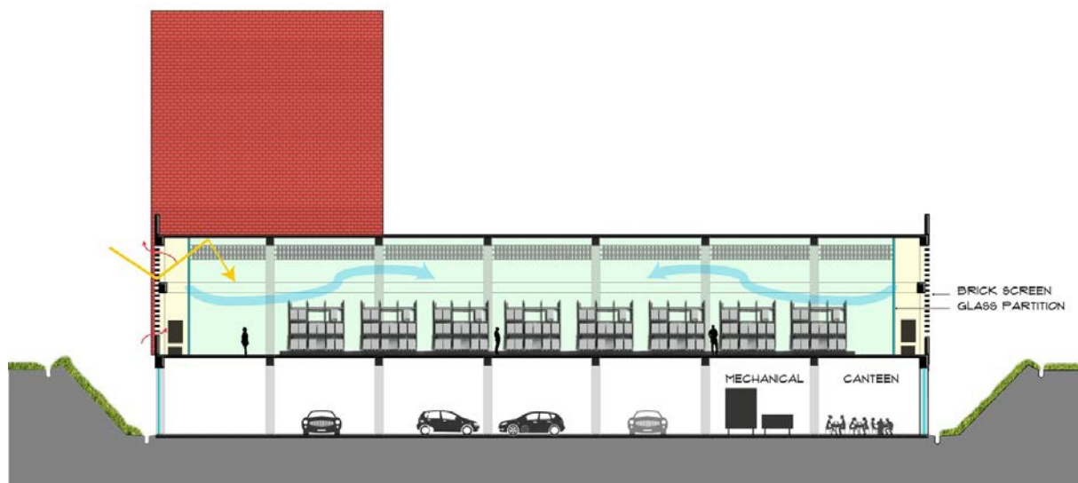
Figure 2 Automated Warehousing Facility Natural ventilation
