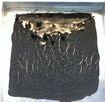
Figure 3.3: Carbon grease polymer composite. After evaporation of the solvent, high carbon grease content caused cracks on the surface.
