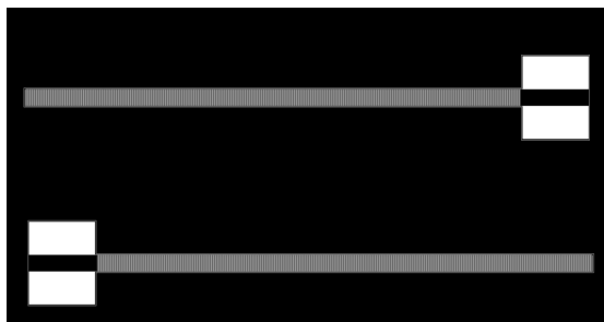
Figure 3.16: Top view of the photomask design used for patterning the photoresist for fabrication method I. The white features are transparent when printed on the photomask and allow the transmission of light onto the photoresist, allowing the illuminated areas of SU-8 to crosslink.
