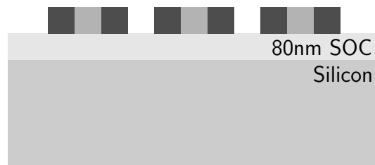
Figure 3.8: Etching of the nitride spacer layer
