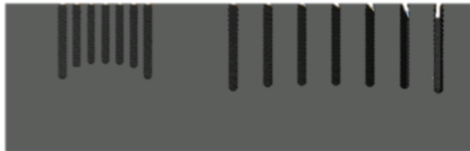
Figure C.4: Affect of microloading for two same-pitch patterns both with the same space size. [97]
