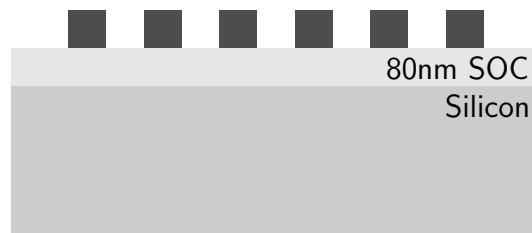
Figure 3.9: Removal of the oxide mandrel
