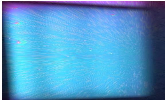
Figure 4.1: SOG coating depicting streaks and comets
