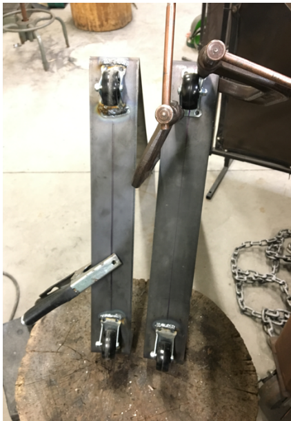
Process of Welding the Wheel and Fixing the Frame onto the Painting
