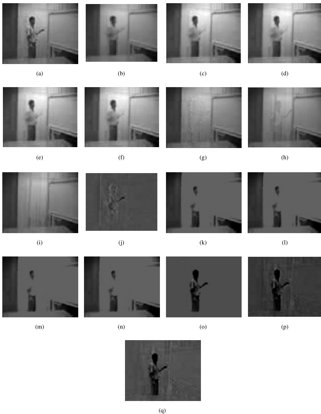
Figure 4.14: Video processing experiment – video 3. (a) Original frame. Background extracted by (b) ISVD [62], (c) GRAFTA [82], (d) PCP [19], (e) OR-PCA [74], (f) RPCA [29], (g) ReProCS [72], (h) method of [47], and (i) L1-IPCA (proposed). Foreground extracted by (j) ISVD [62], (k) GRAFTA [82], (l) PCP [19], (m) OR-PCA [74], (n) RPCA [29], (o) ReProCS [72], (p) method of [47], and (q) L1-IPCA (proposed).
