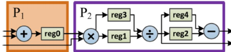
Figure 3.3: Example Pipelined Architecture [5]
