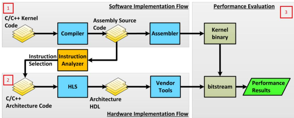
**Figure 3.1:** Flow diagram of Customized Soft Processor[4]
