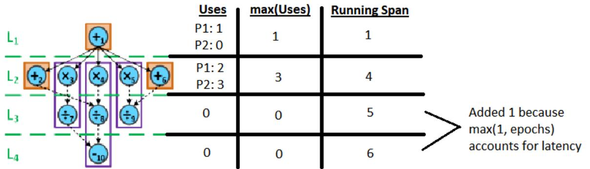
Figure 4.1: Example of Span Determination
