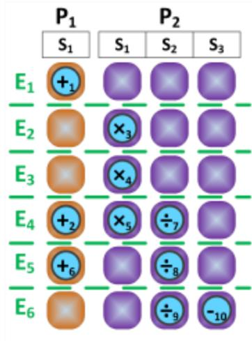
**Figure 3.7:** Example Pipelined Architecture Execution Schedule (E - Epoch) [5]
