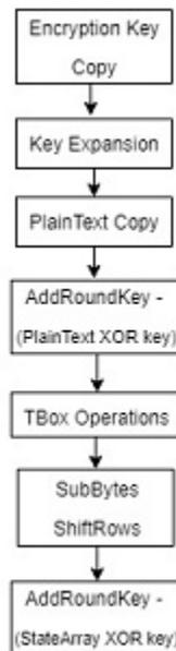
**Figure 4.5:** High Level Dataflow Graph of AES with TBox
