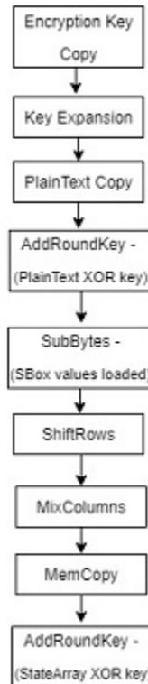
**Figure 4.4:** High Level Dataflow Graph of AES
