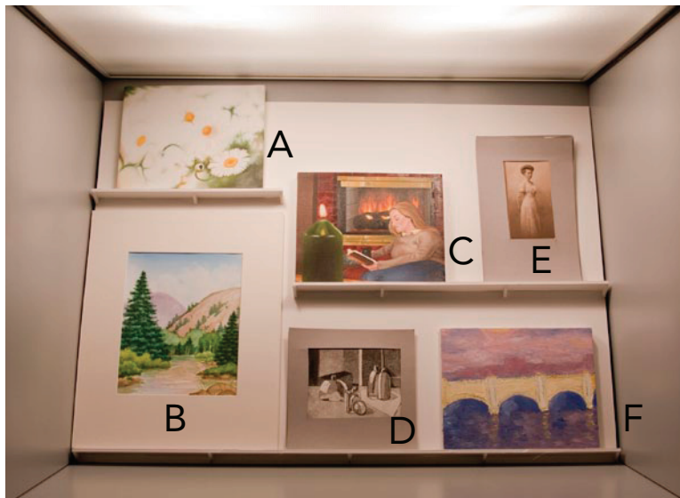
Figure 15. Experimental viewing setup with the Macbeth Spectralight III light booth, illuminated by source 'A,' used to acquaint observers with the original works of art 13
