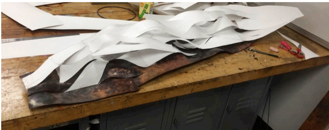
Figure 24. First layer of copper sheet with second and third layers of paper model.
