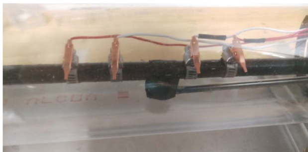
Figure 36. Photograph of 4 electrical probes mounted inside the glass cylinder test chamber.
