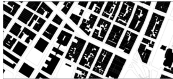
Figure ground map of lower Manhattan showing positive and negative space.
