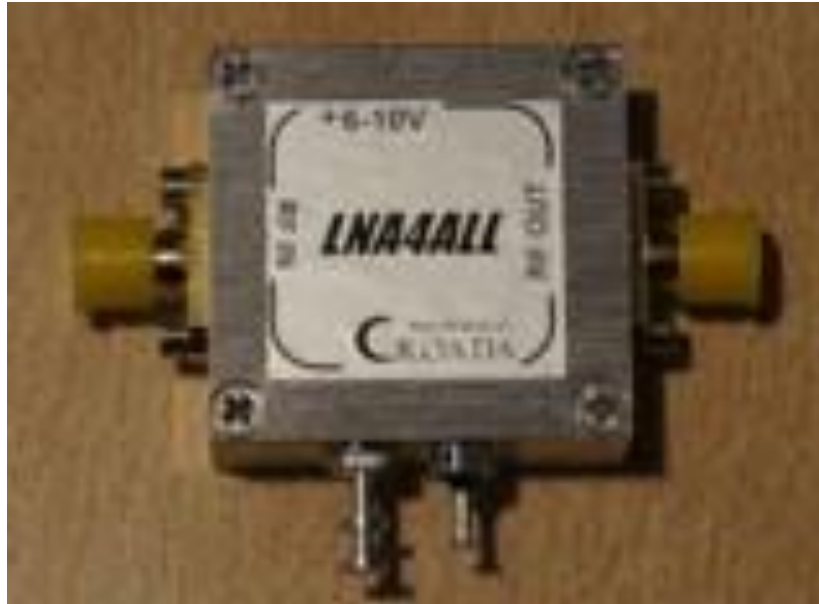
Figure 13: Low Noise Amplifier with gain of 23.5dB @VHF frequencies
