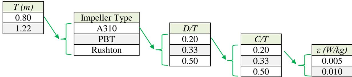
**Figure 6.2.1. An example of progressions through the five variables (Tank diameter,  $T$ , impeller type,  $R$ , impeller to tank diameter ratio,  $D/T$ , impeller off-bottom distance to tank diameter ratio,  $C/T$ , and the mean energy dissipation rate,  $\epsilon$ ) and their respective levels.**
