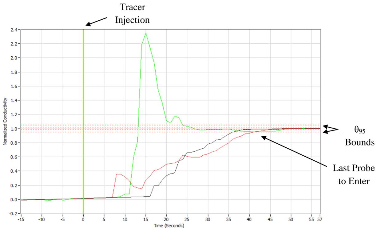
**Figure 5.2.3. Example of  $\theta_{95}$  determination using normalized conductivity responses at a sampling rate of 1 s from SPX Flow Lightnin’s custom LabVIEW blend time application for three probes.**
