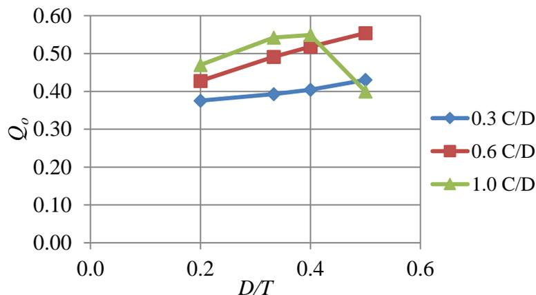
**Figure 5.1.3. Effect of impeller diameter to tank diameter ratio,  $D/T$ , and impeller off-bottom distance to impeller diameter ratio,  $C/D$ , on the flow number,  $Q_o$ , produced by a Lightnin A310 impeller geometry in a 1.22 m diameter baffled tank from a CFD simulation based study.**
