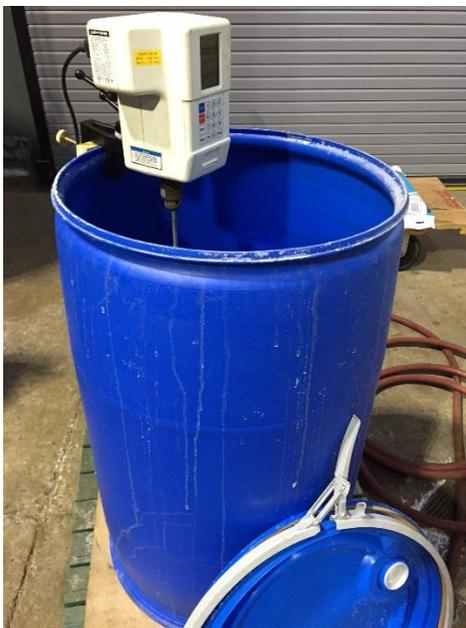
**Figure 6.4.2. Tracer make down apparatus composed of a 208 L barrel and clamp-mounted SPX Flow Lightnin Labmaster agitator. Photo courtesy of SPX Flow Lightnin.**
