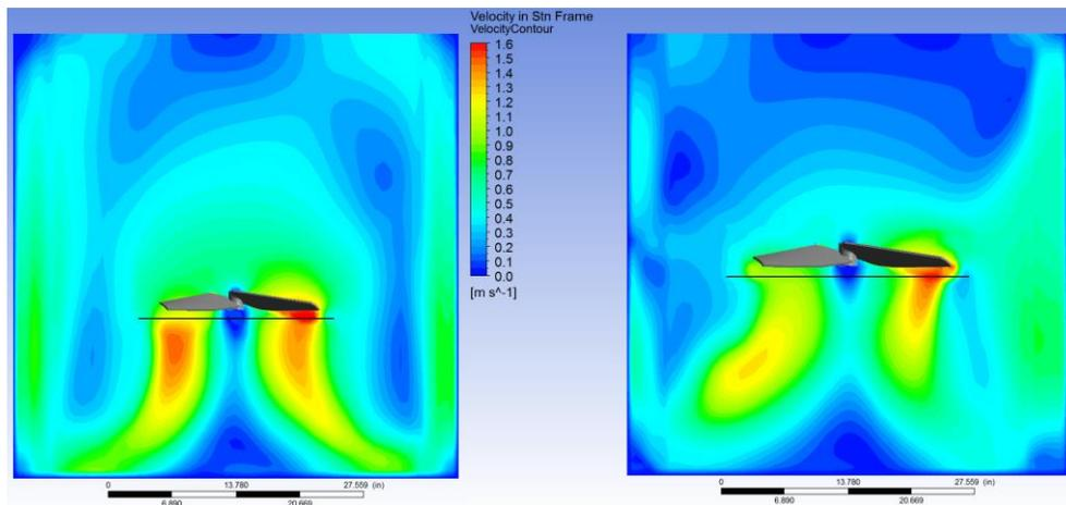
**Figure 5.1.4. Velocity contour plots for a cross-section of the vessel for an optimum case (impeller diameter to tank diameter ratio,  $D/T = 0.4$ , and impeller off-bottom distance to impeller diameter ratio,  $C/D = 1$ ) and outlier case ( $D/T = 0.5$  and  $C/D = 1$ ) from left to right with the black line under each impeller designating the region of primary flow.**
