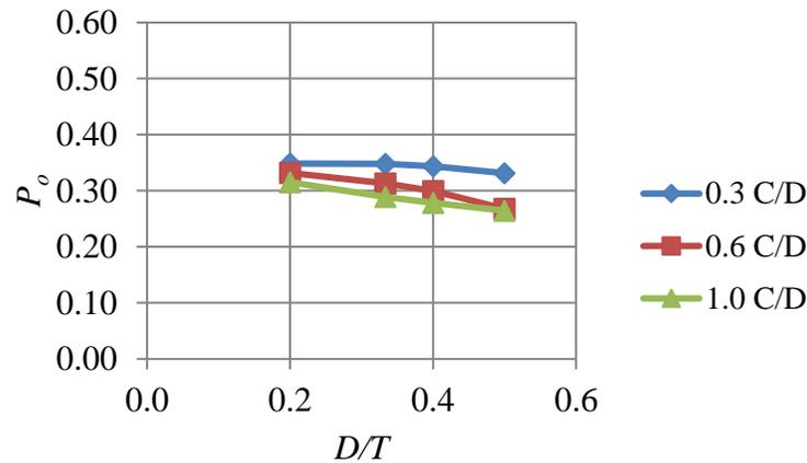
**Figure 5.1.2. Effect of impeller diameter to tank diameter ratio,  $D/T$ , and impeller off-bottom distance to impeller diameter ratio,  $C/D$ , on the measured power number,  $P_o$ , of a Lightnin A310 impeller geometry in a 1.22 m diameter baffled tank from a CFD simulation based study.**
