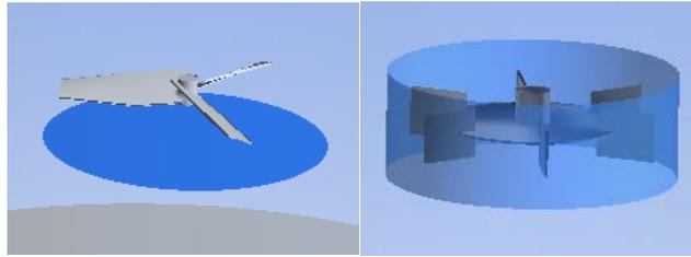
**Figure 3.2.2. Depiction of primary flow measurement area for axial flow impellers (left) and radial flow impellers (right). The primary flow area is defined by the swept area for axial impellers (left) and a tangential ring for radial flow impellers (right). Visualization courtesy of SPX Flow Lightnin.**
