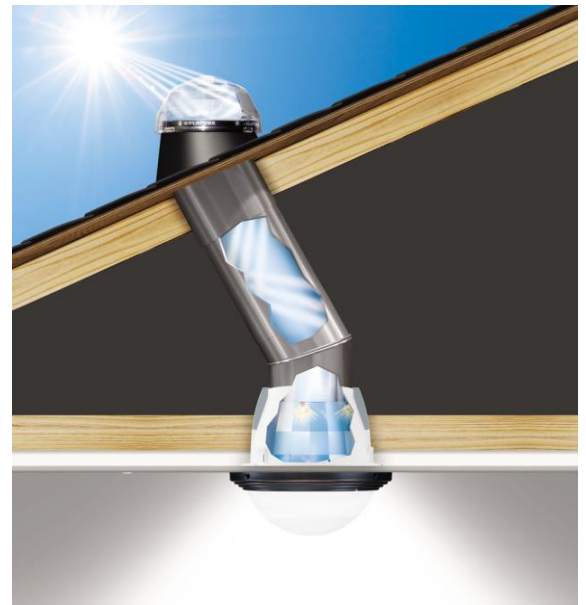
Figure 4. Example of Solartube or Lighttube http://netzeromax.com/solatube-introduces-the-new-solatube-smart-led-system/
