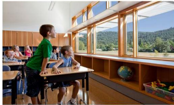
Figure 10. Light Shelf in Classroom at Thurston Elementary School, Designed by Mahlum https://www.disd.edu/blog/daylighting-interior-design/
