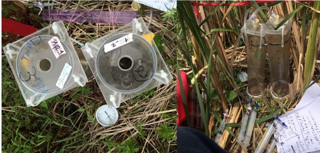
Figure 5. Field measurement of soil respiration using small chambers.
