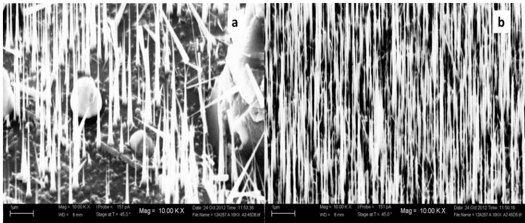
Figure 5.7 45° degree tilted SEM image of InAs NW with Au thermal evaporation (a) patterned (b) un-patterned.
