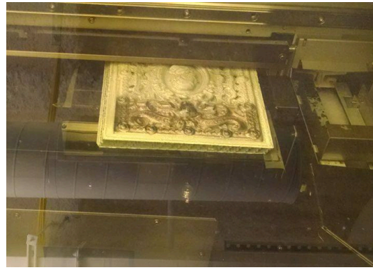
Figure 15: Printing on the VersaUV ink cured printer, photos by author.
