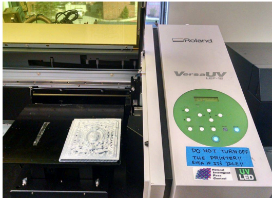
Figure 15: Printing on the VersaUV ink cured printer, photos by author.
