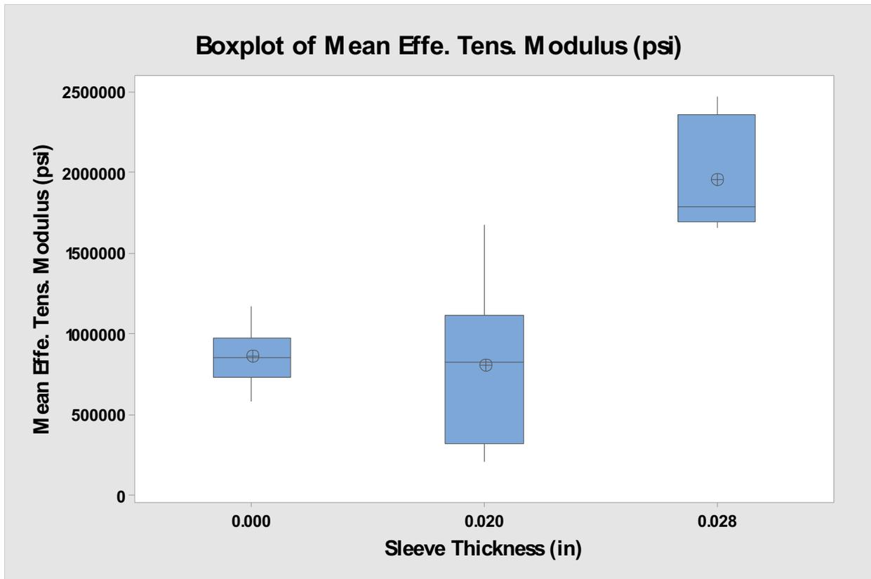
*Figure 7.43: Boxplot of tensile modulus for each sleeve thickness factor level.*
