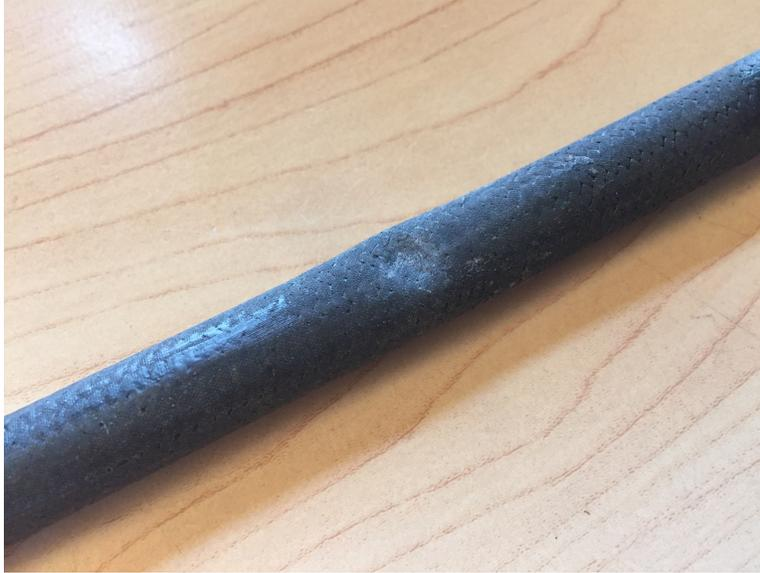
*Figure 12.101: Impact site of 0.028 sleeve thickness post impact sample.*
