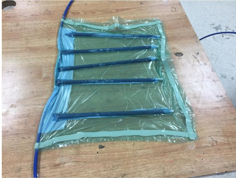
*Figure 7.9: Vacuum bagging system used for composite sleeve manufacture.*
