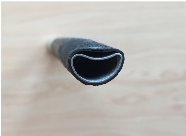
*Figure 7.55: 0.020 sleeve thickness factor level post impact cross section.*
