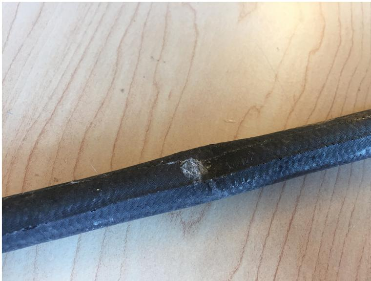
*Figure 12.98: Impact site of 0.020 sleeve thickness post impact sample.*
