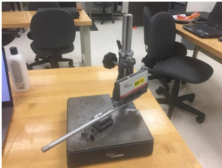
*Figure 12.2: Surface roughness testing of aluminum sleeve using Mahr Federal Pocket Surf.*
