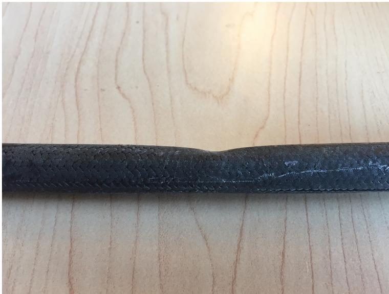
*Figure 12.100: Profile of 0.028 sleeve thickness post impact sample.*
