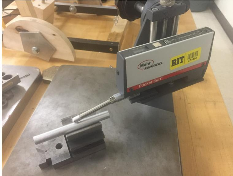
*Figure 7.4: Surface roughness testing of aluminum end using Mahr Federal Pocket Surf.*
