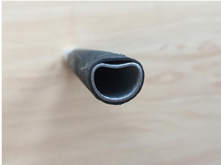
*Figure 7.56: 0.028 sleeve thickness factor level post impact cross section.*
