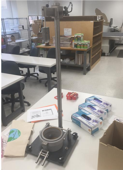
*Figure 7.17: Original drop impact tester before modifications.*
