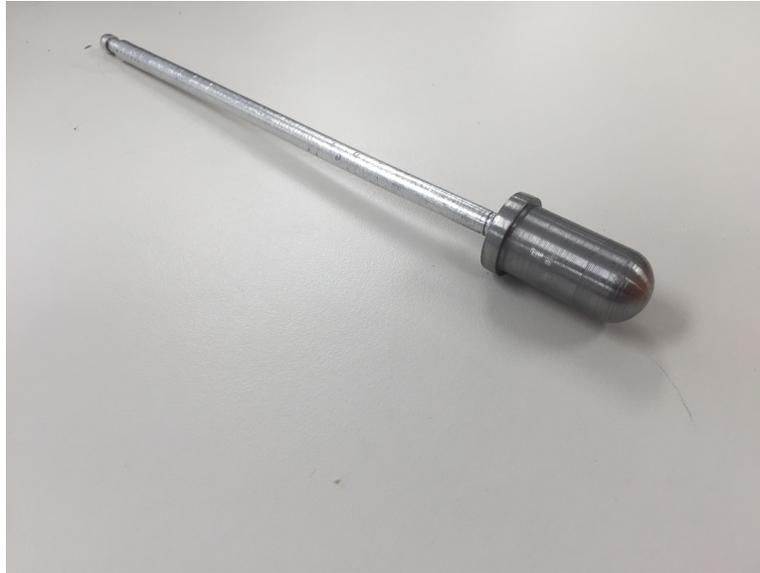
*Figure 7.19: Impactor as machined, not including necessary weights.*
