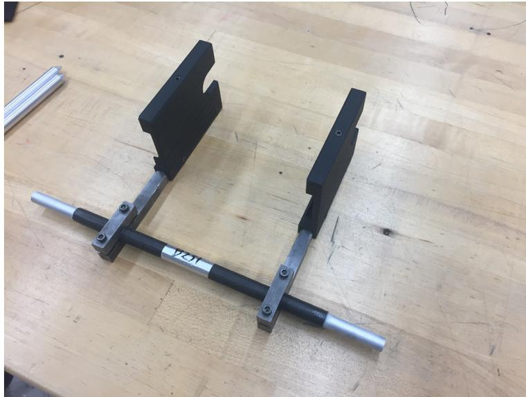
*Figure 7.16: Assembled sleeve, with inclinometer fixture in place.*
