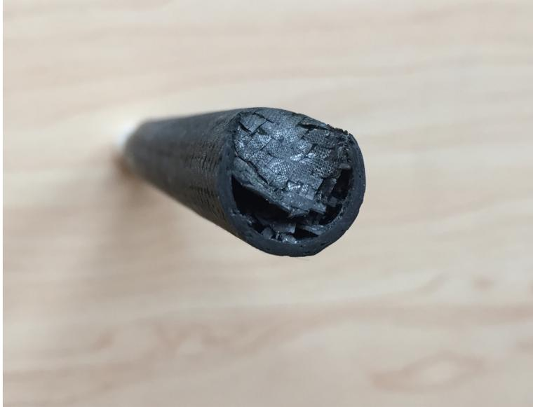
*Figure 7.54: Non sleeve (0.000 sleeve thickness factor level) post impact cross section.*
