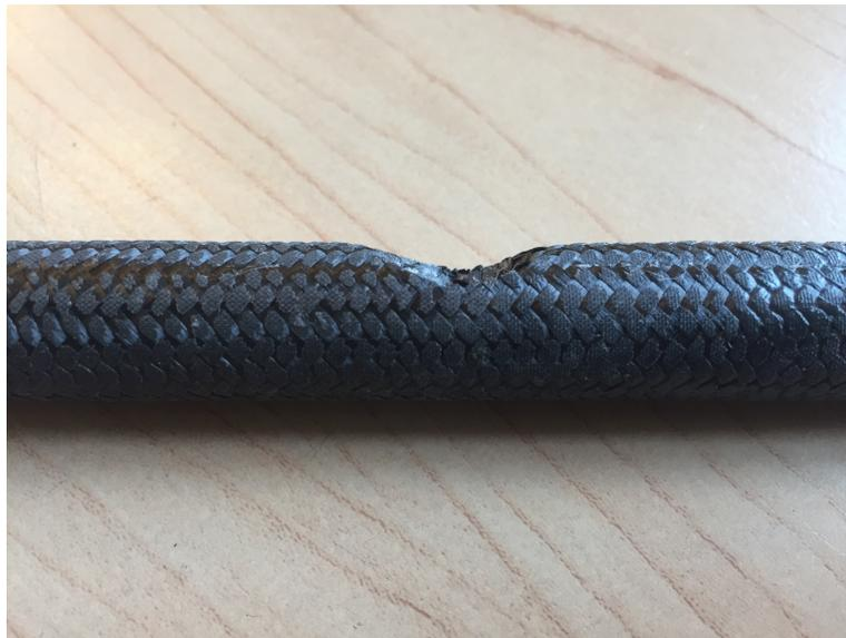
*Figure 12.94: Profile of non sleeve post impact sample*
