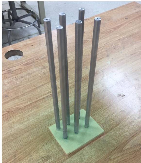
*Figure 7.8: Fixture used to spray mandrels in an even manner.*
