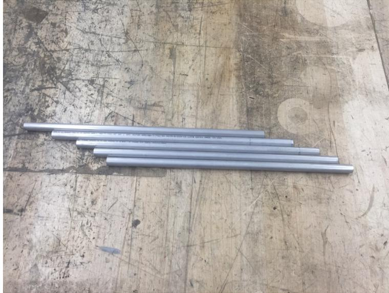
*Figure 12.1: Aluminum sleeves, machined to their final length.*
