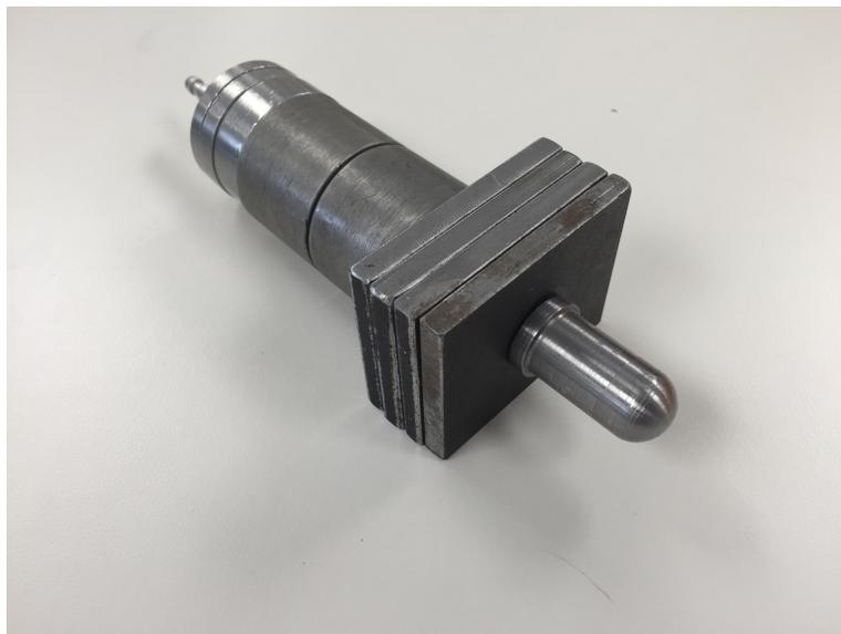
*Figure 7.20: Impactor including necessary weights.*
