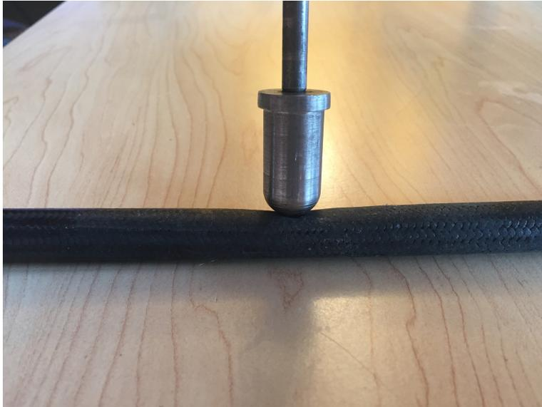
*Figure 12.99: Impactor overlap of 0.028 sleeve thickness post impact sample.*
