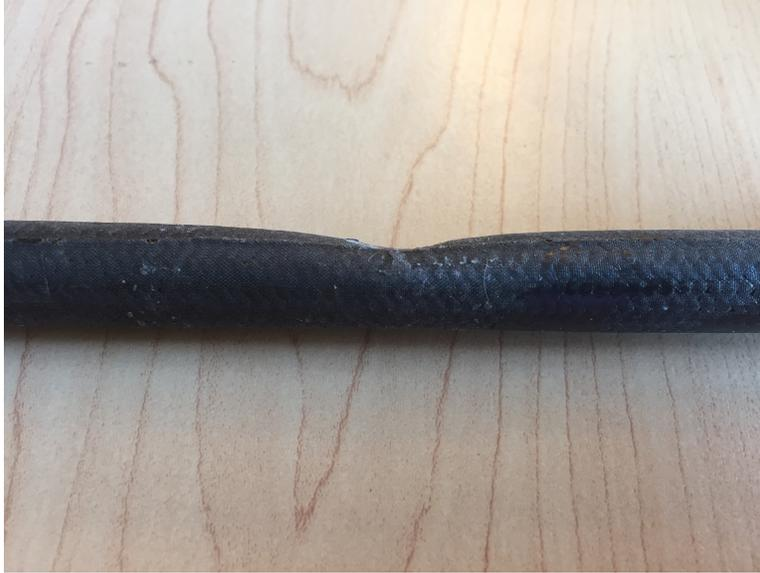
*Figure 12.97: Profile of 0.020 sleeve thickness post impact sample.*
