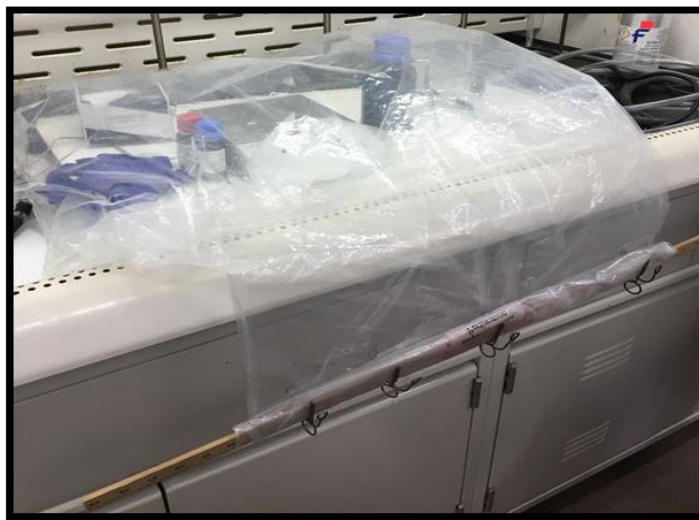
Figure 6.5: Glove bag sealed and partially filled with inert gas
