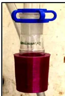
Figure 6.9: PLA printed sleeve for glass joint
