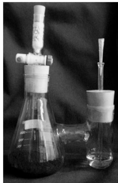
Figure 2-4. Setup of a biometer flask used for CO 2 evolution determination (Gonçalves and Franchetti 2015).
