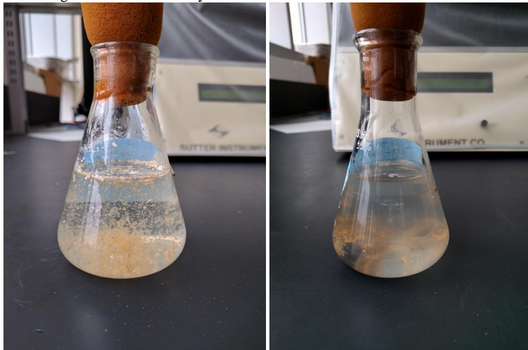
Figure 2-9. CPZ-6A cultures grown in Bushnell-Haas broth. Cultures were grown with low (left, 62mM) and moderate THF (right, 616mM). Note fungal colony in bottom left of the right flask- fungus has been seen only in this enriched culture
