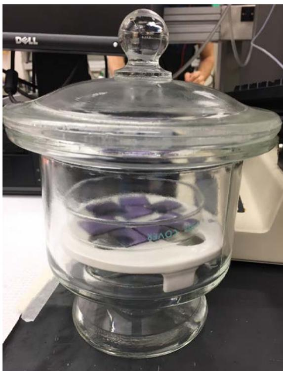
**Figure 7.1: Solvent Vapor annealing set up**
