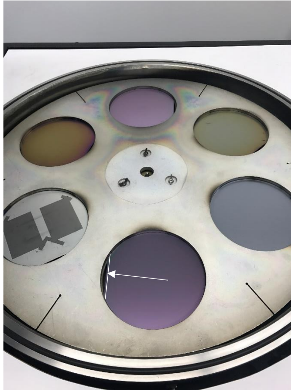
Figure 3.4. Alignment of wafer flat to the left in sputtering chamber platen.
