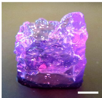
Figure 30 An image of a 3D printed tubular structure using 50% (v/v) Matrigel and 3 wt% agarose. The tube has a diameter of 17 mm and a wall thickness of 2 mm (scale bar: 5 mm).
