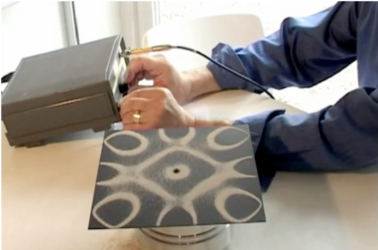
Figure 18: Cymatics Sand Vibration Plate
