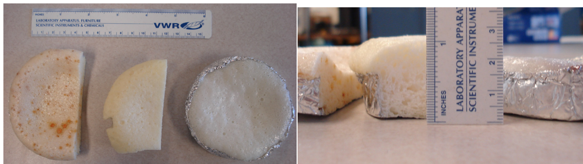
Figure 11- foam samples names left to right EXOCHEM10, ENDOCHEM10 and ENDOPHY10 respectively
