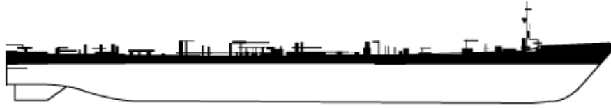
Fig. 1.4. Coastal ocean tank barge. Designed to carry petroleum products. 550 ft. long, 225,000-barrel capacity (1 barrel = 42 gallons).
